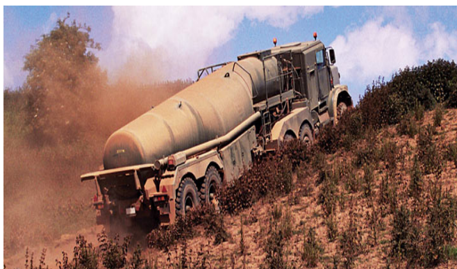
Figura Nro 29 MTVR CST (Close Support Tanker)
