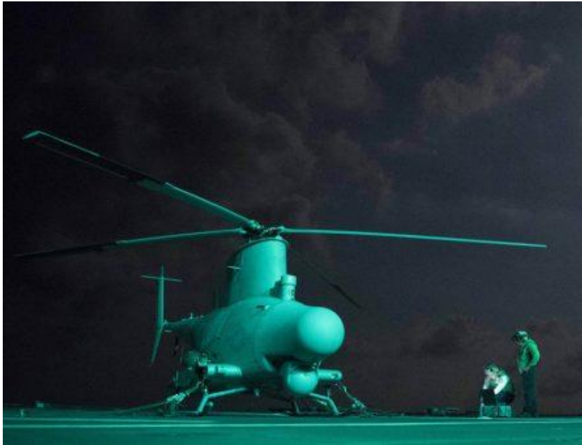
Fig. 43. The MQ-8B Fire Scout is based on Schweizer aircraft model 330. U.S. Navy.
