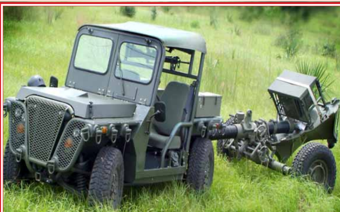
ITV – EFSS PM (Internally Transportable Vehicle – EFSS Prime Mover) transportando el mortero de 120mm.
