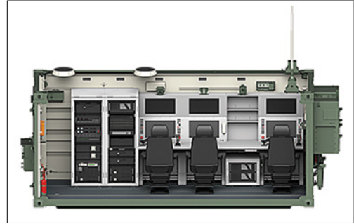
FIGURA 25: BAYRAKTAR TB-2 GROUND CONTROL STATION
