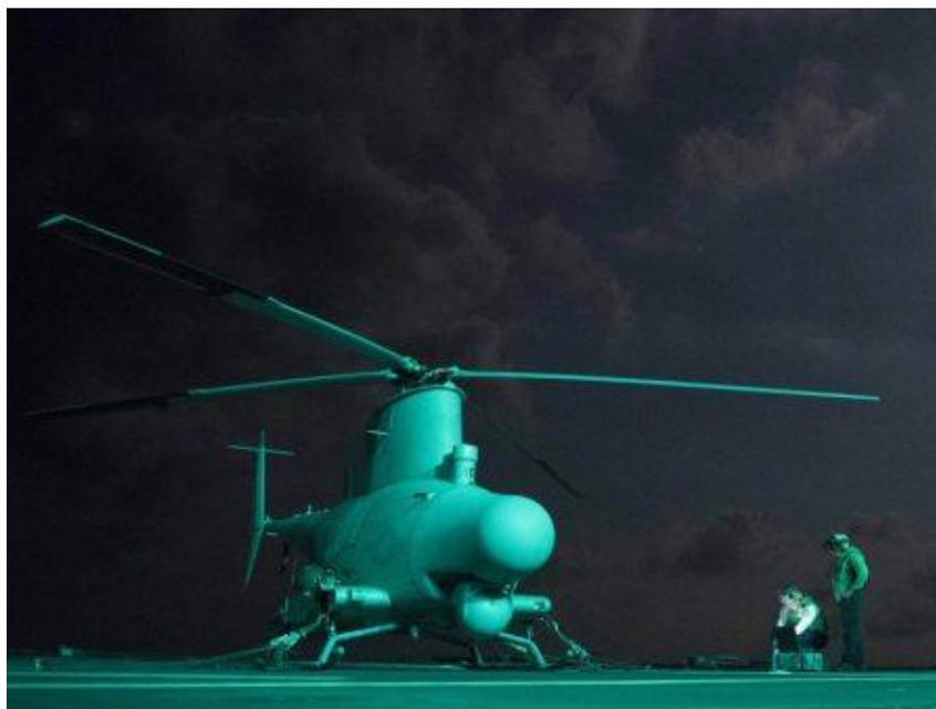
Fig. 50. The MQ-8B Fire Scout is based on Schweizer aircraft model 330. U.S. Navy.
