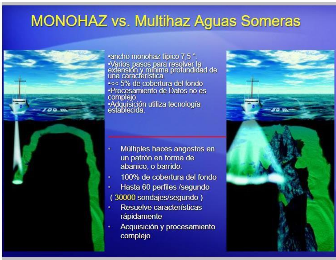
Figura 5.8 Comparación monohaz vs multihaz- https://slideplayer.es/slide/3813789/#google_vignette
